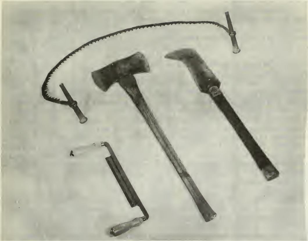
Figure 10.--Girdling tools used in high release of planted conifers. Draw shave (on left), double-bit axe, Phelps tool (right), and girdling chain saw (at top).
